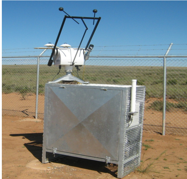
Fig. 2: DNI measuring station (wind and temperature sensor not shown)
