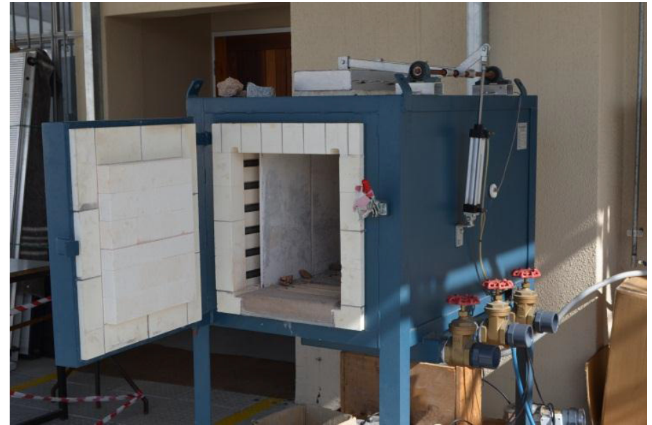
Fig. 1 KILN oven for testing samples up to 1000 °C
