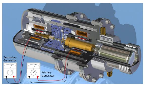
Hermetically sealed, filled with helium under pressure
