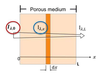
To determine the absorption coefficient
