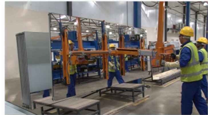
The Rioglass factory in Upington manufactures the panels for the Khi heliostats and employs some 80 local people
