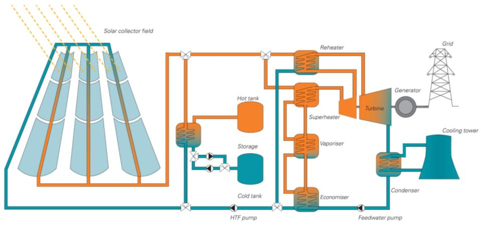
Parabolic trough power plant – thermal flow
