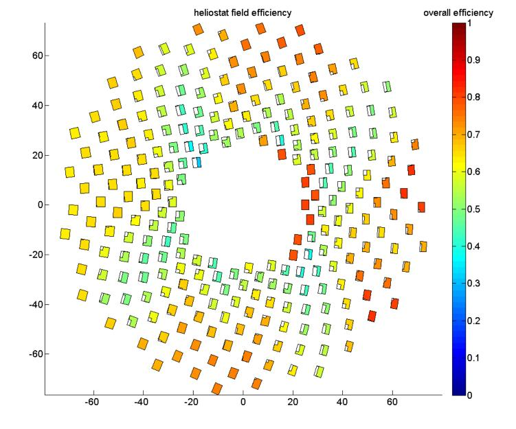
SBP Solar field efficiency – blocking and shading optimisation
