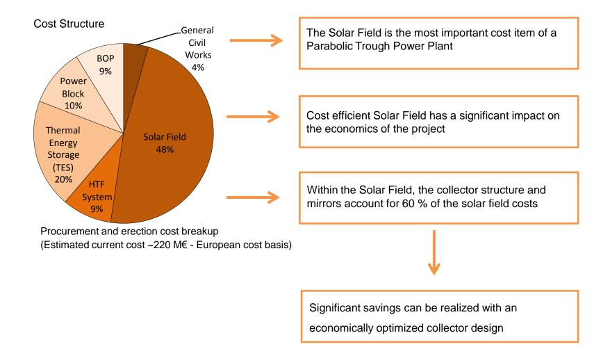
Cost efficient solutions for parabolic trough power plants: An economically optimized collector design is a key to reduce CSP project costs
