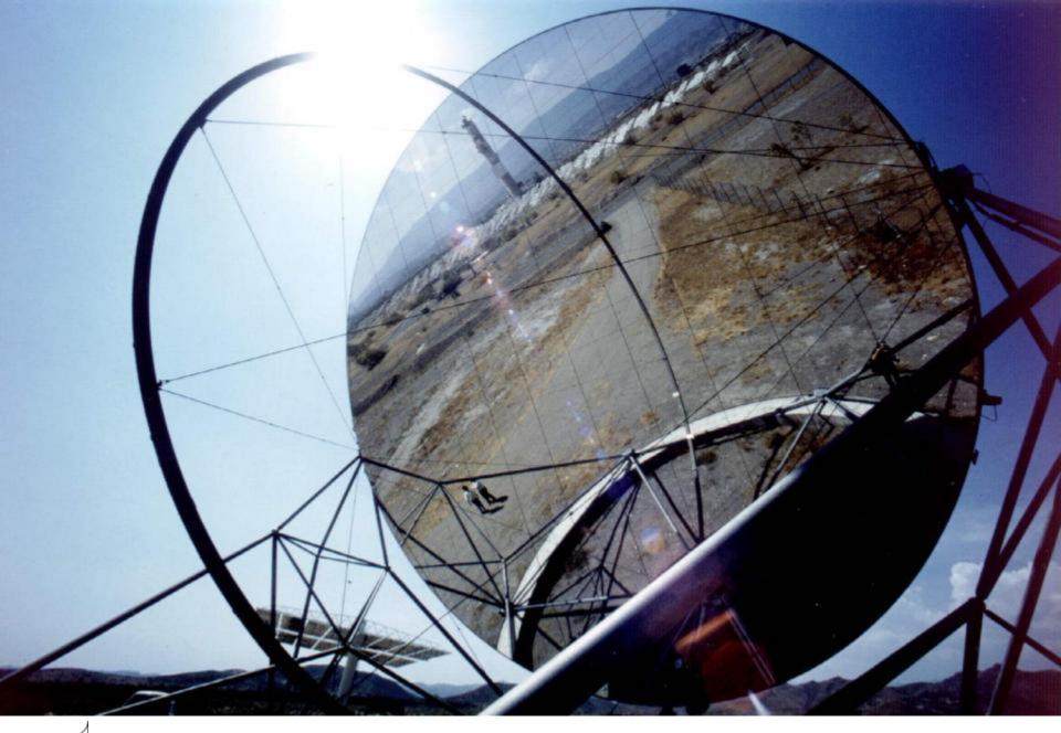
SBP / Steinmüller 150 m<sup>2</sup> metal membrane heliostat – optical quality
