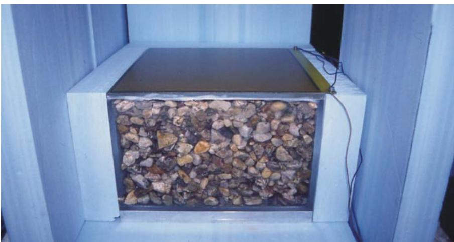
⌚ Test rig for effective heat conduction
