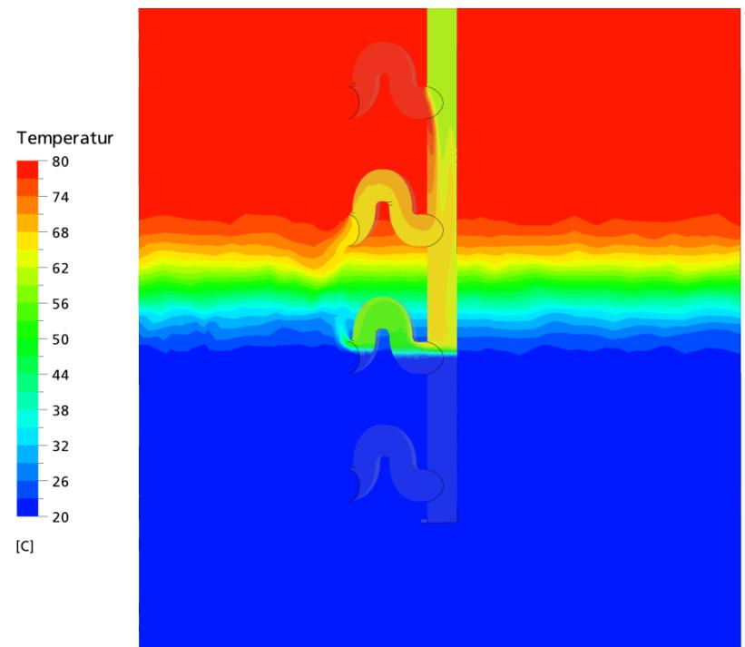
① Development and analyse of a lance for stratification with CFX,
