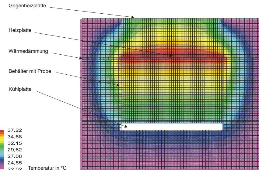
⌚ Recalculating with CFX, 3D, temperature
