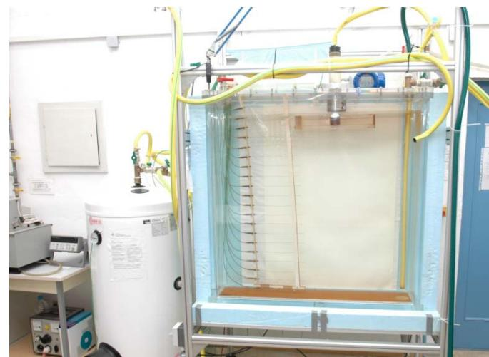
Plexi 1\* – Test rig for visualization of flow
