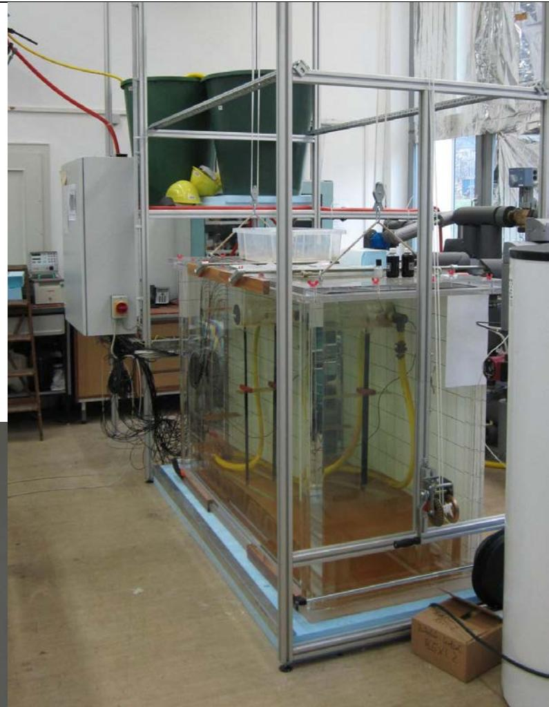
➊ Test of a slotted pipe diffusor
