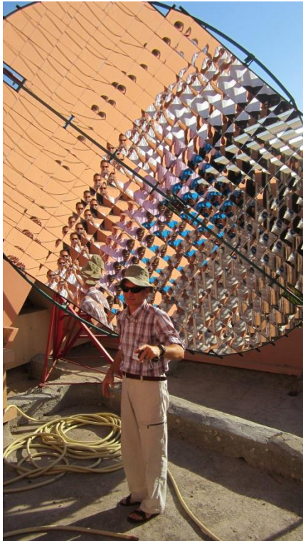
Wolfgang Scheffler demonstrating a Scheffler reflector at the local university. (Photo: Paul Gauché)
