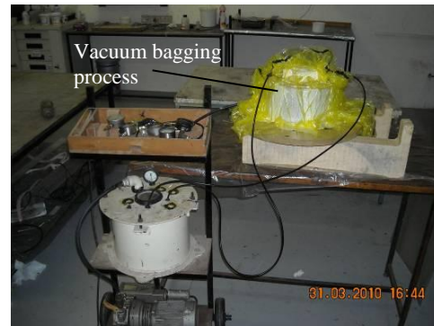
Fig. 3. Pre-vacuum bagging process showing the Miro 4 aluminum attached to the paraboloidal mold. Glass and carbon fibre profiles were hand impregnated with resin for the hand lay-up process (left). A vacuum bag is applied to improve consolidation and allow for additional pressure forming of the aluminum on to the paraboloidal mold.
