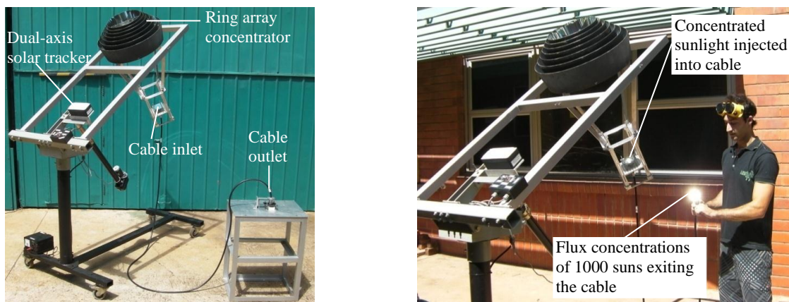
Fig. 2. FOCUS consisting of a ring array concentrator integrated with a fibre optic cable to provide high-flux levels remote from the collector (left). FOCUS in operation, concentrating incoming solar rays into a fibre optic cable (right).
