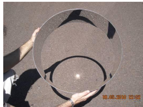
Fig. 4. After the vacuum-bagging process is completed the completed FRP element is detached using tabs (left). A completed reflective element focusing incident rays to a point (right).
