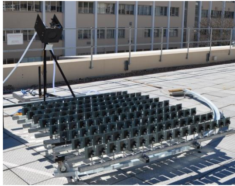
Fig. 6. Experimental layout of the small-scale 1.5 kW heliostat field, comprising 150 flat mirrors mounted on a manual, dual-axis rotating framework.
