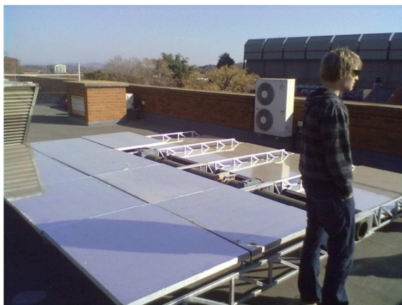
Figure 1: Big heliostat (25 m 2 ) mirror frame
