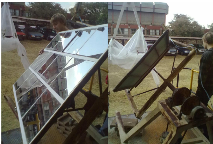
Figure 6: Small heliostat (1.08 m 2 )
