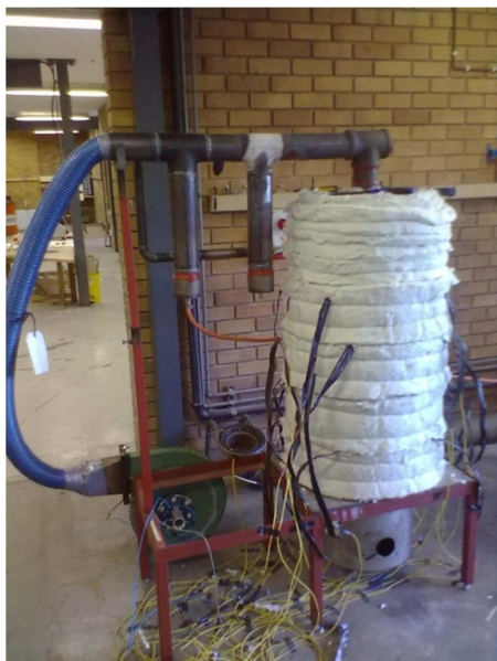
Figure 9: Packed bed thermal storage experiment
