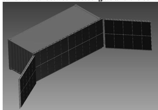
**Figure 7: 'Book-style' - The security gates swing open revealing the solar panels**
