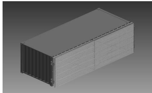
**Figure 6: 'Book-style' - Solar panels are securely sandwiched between a steel gate and the container**
