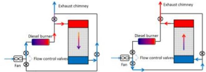
Fig. 4. Schematic of air flow direction in the TES test rig.
