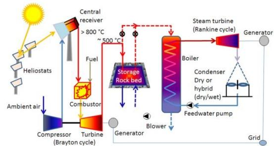
Fig. 1. SUNSPOT cycle solar power plant schematic [2].
