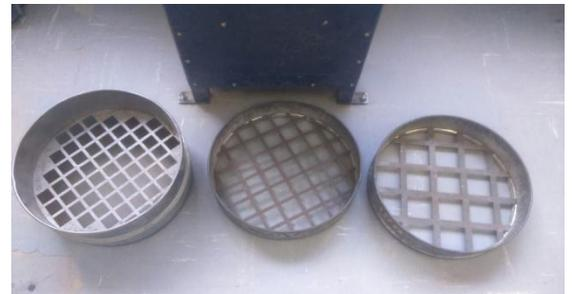
Fig. 6. Automatic Sieving machine with different sized sieve sheets for size classification of granular materials.
