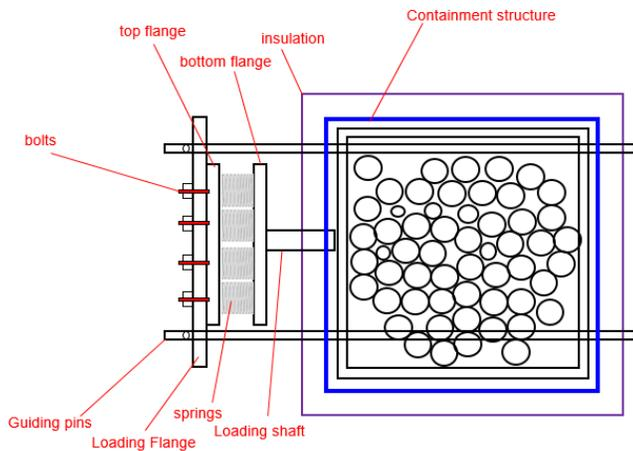
Fig. 5. Test Rig schematic for combined mechanical and thermal loading of packed rock bed.
