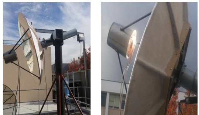
Fig. 7: Parabolic dish and conical receiver set up
