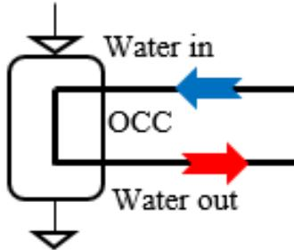
$$T_{cwo} = \frac{Q_{max}}{\dot{m}_{cw} c_{p,cw}} + T_{cwi}$$
