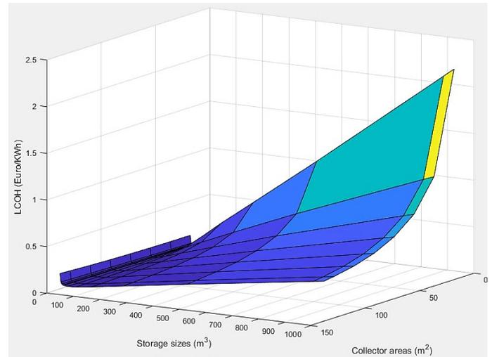
**Fig. 7. Plot of LCOH vs Collector areas and storage sizes**
