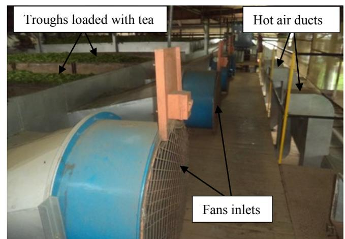
Fig. 1. Withering system set-up
