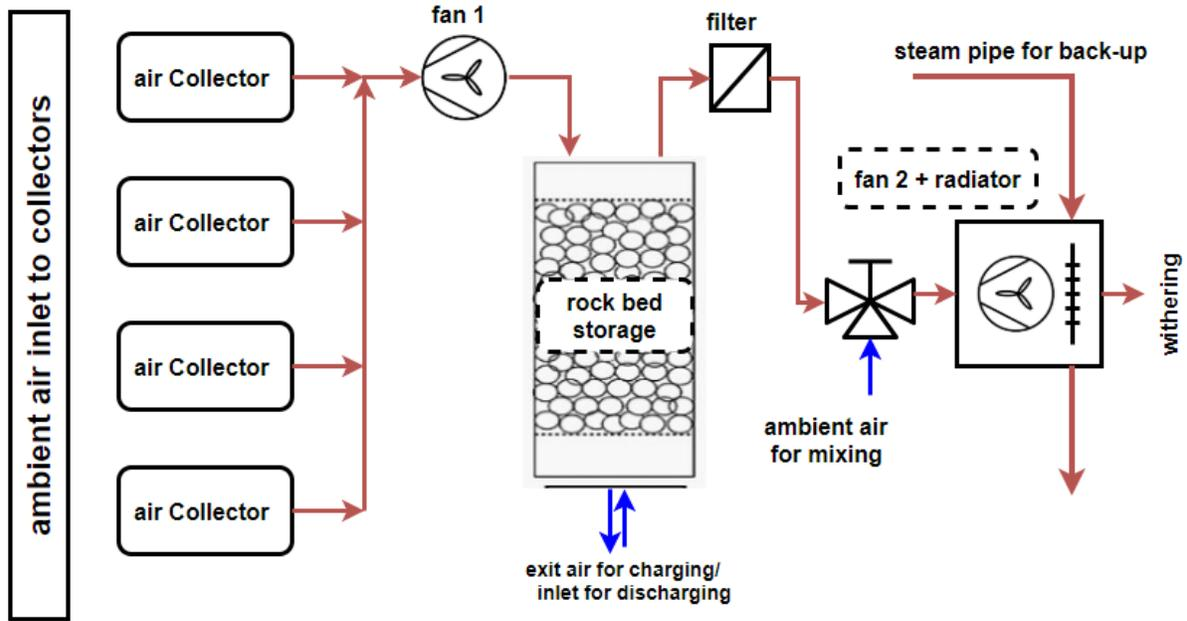
Fig. 5. Schematic diagram of the solar air system
