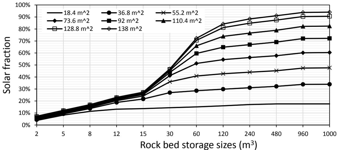
Fig. 6. Plot of solar fraction vs storage size for 8 different collector areas
