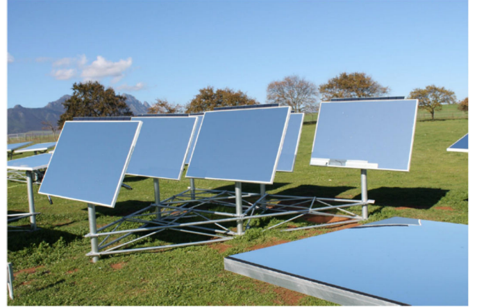
Fig. 6: Photograph of a HeliPod while tracking
