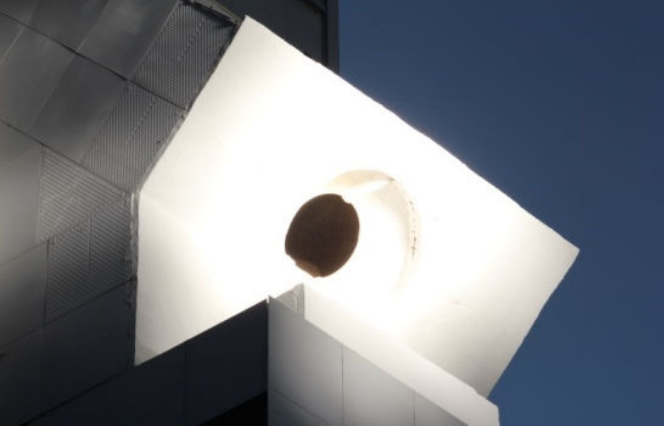
Fig. 10: Receiver in operation [10]
