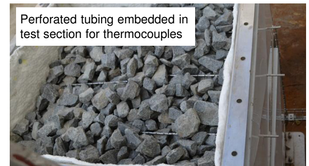
Fig. 2 Insulated storage vessel packed with test material
