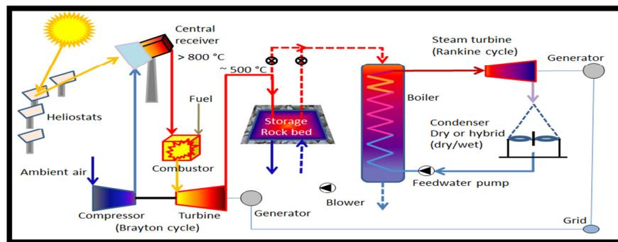
Figure 1: Representation of Basic SUNSPOT cycle [1]
