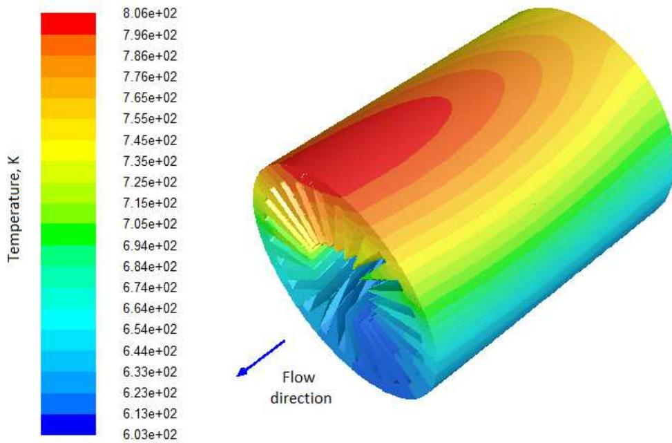
**Figure 3.** Temperature contour plots on solid surfaces.
