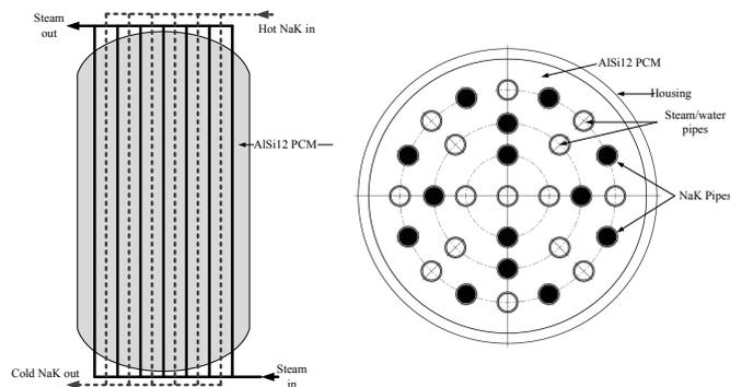
**Figure 3–Metallic phase change thermal storage concept**
