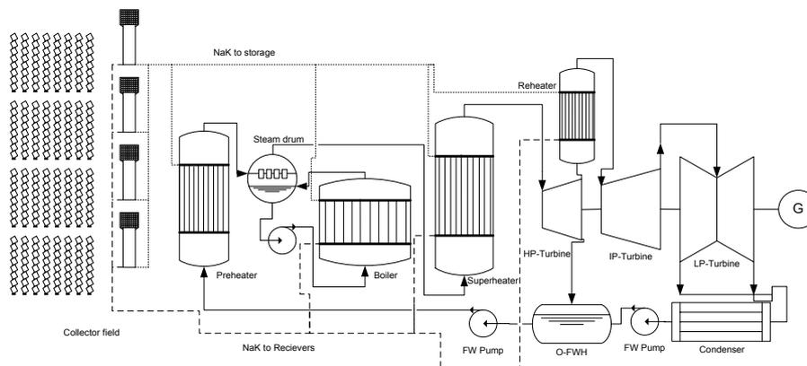
**Figure 4 - NaK in a steam cycle**
