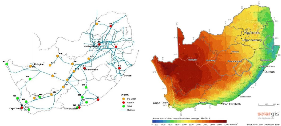
**FIGURE 1.** (a) WWF nodes located near existing HV transmission lines. (b) DNI map of South Africa (GeoModel Solar 2014).
