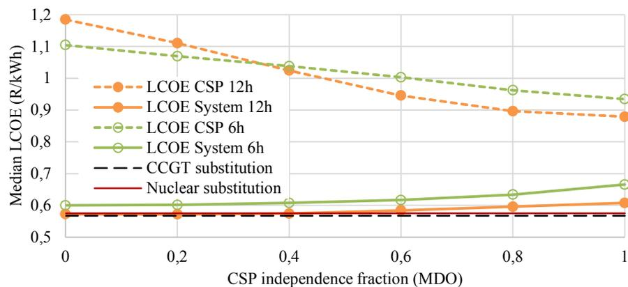
**FIGURE 6.** LCOE of the CSP fleet and the whole system for CSP plants with 6 or 12 storage hours as a function of system independence (or MDO). An MDO of zero implies that the CSP fleet serves only a system availability function.
