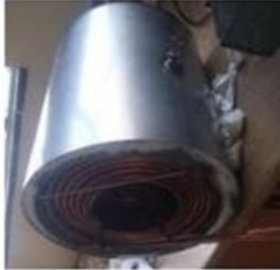
**FIGURE 4.** Manufactured cavity receiver
