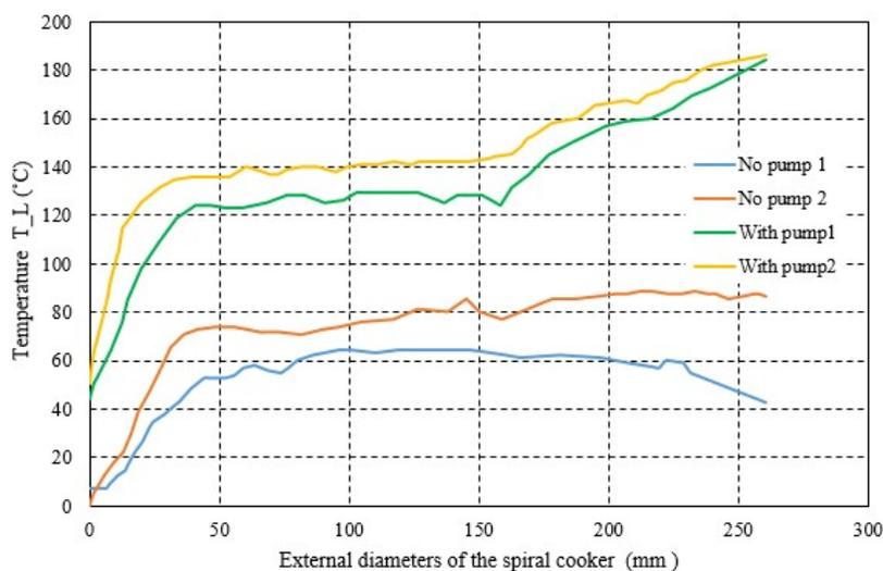
**FIGURE 8.** Average day temperature measured at various diameter of the spiral cooker
