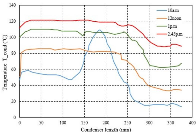
**FIGURE 7.** Wall temperature as a function length of inlet manifold of the condenser of the heat pipe
