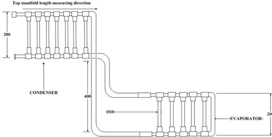
**FIGURE 6.** Heat pipe with condenser and evaporator dimensions
