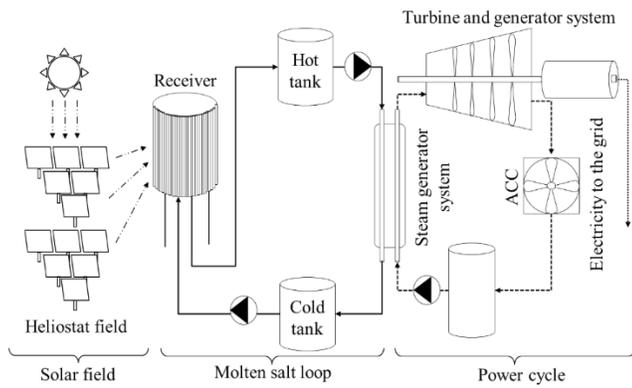
**Fig. 1. Simplified schematic diagram of a molten salt central receiver system**
