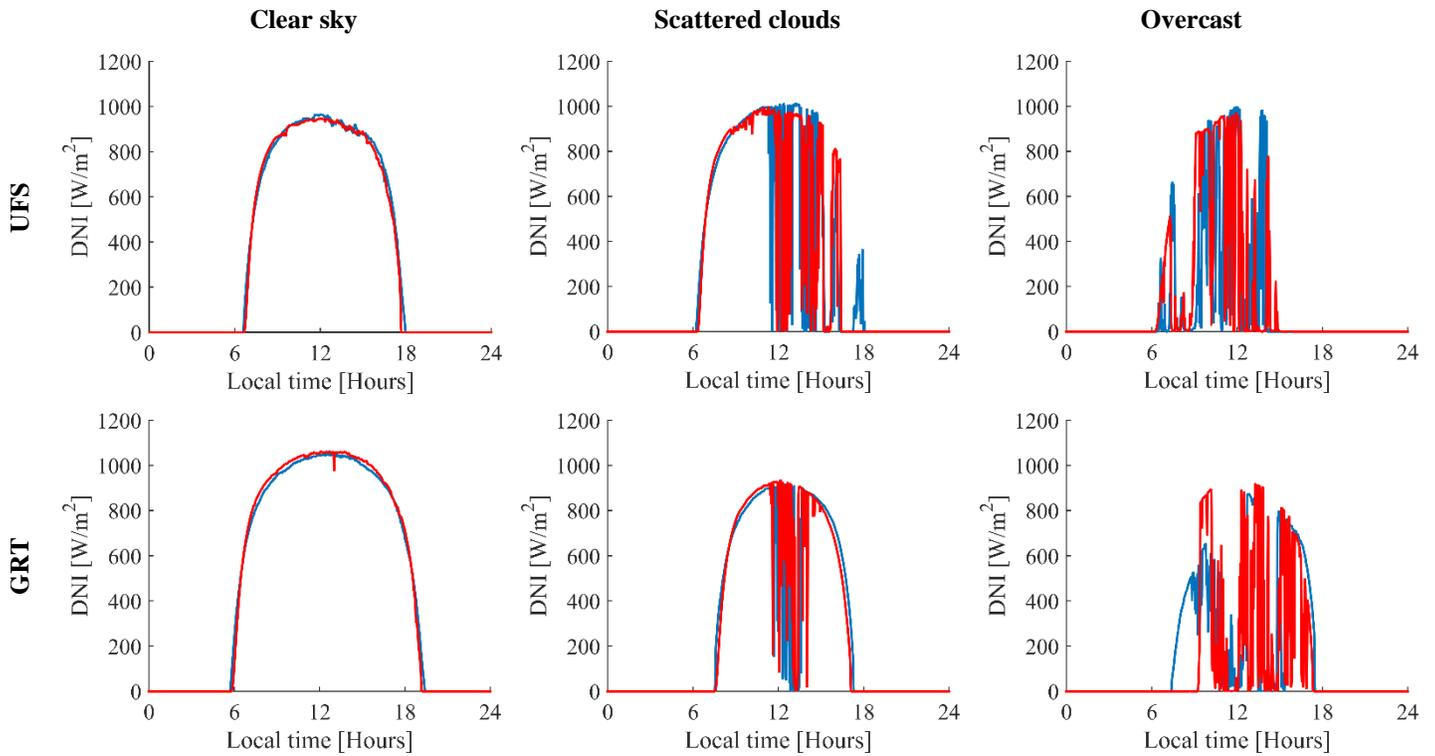
**Fig. 3. Comparison of synthetically generated (red) and measured (blue) DNI curves**
