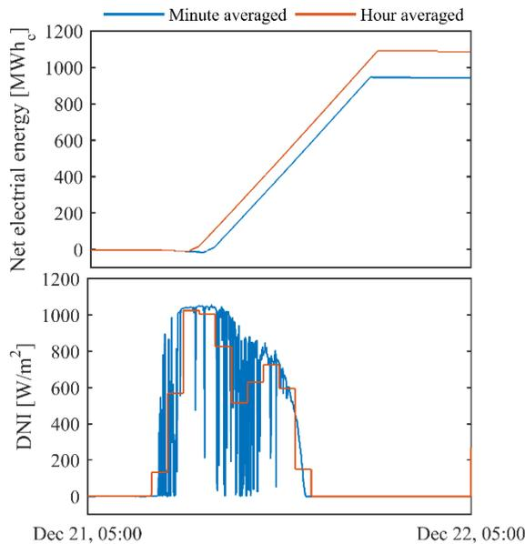
**Fig. 2. The effect of hour vs minute averaged DNI data on the performance of a central receiver model over one day of operation**
