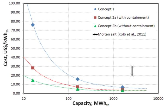
**Fig 3: Cost comparison of different thermal energy storage concepts. Concepts 1 and 2 are both for a packed rock bed as the storage medium [7].**
