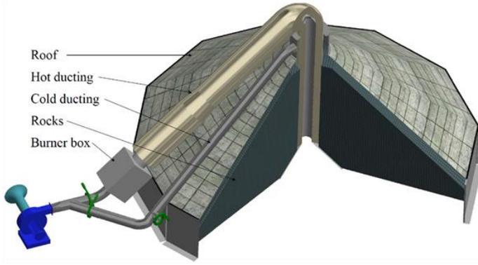
**Fig 1: Cut out drawing of the experimental design**
