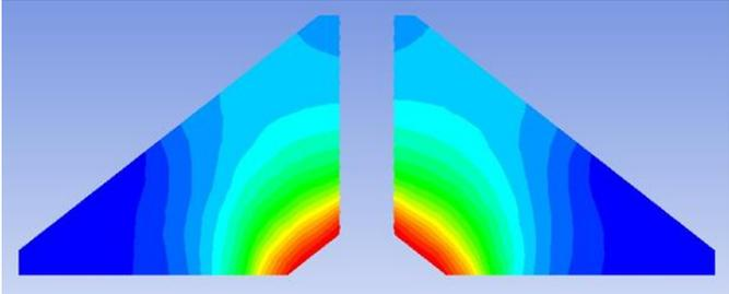
**Fig 4: Qualitative temperature distribution in the packed rock bed, results produced with ANSYS Fluent**
