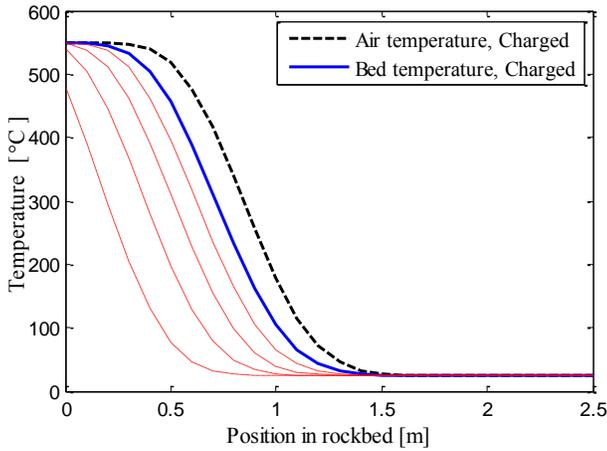
**Fig 2: Temperature distribution prediction over packed bed showing the hourly progression lines of the charging**
